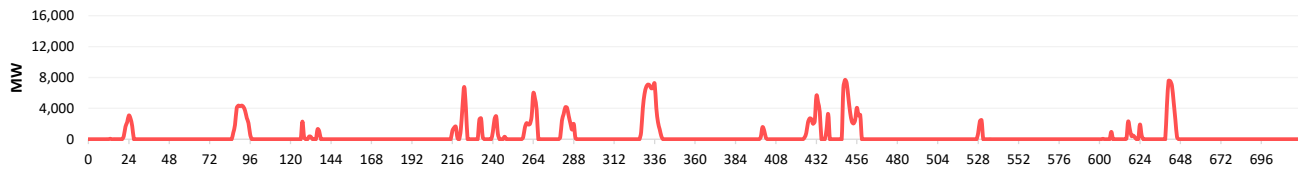
Battery Energy Storage Deployed During Modeling Period
